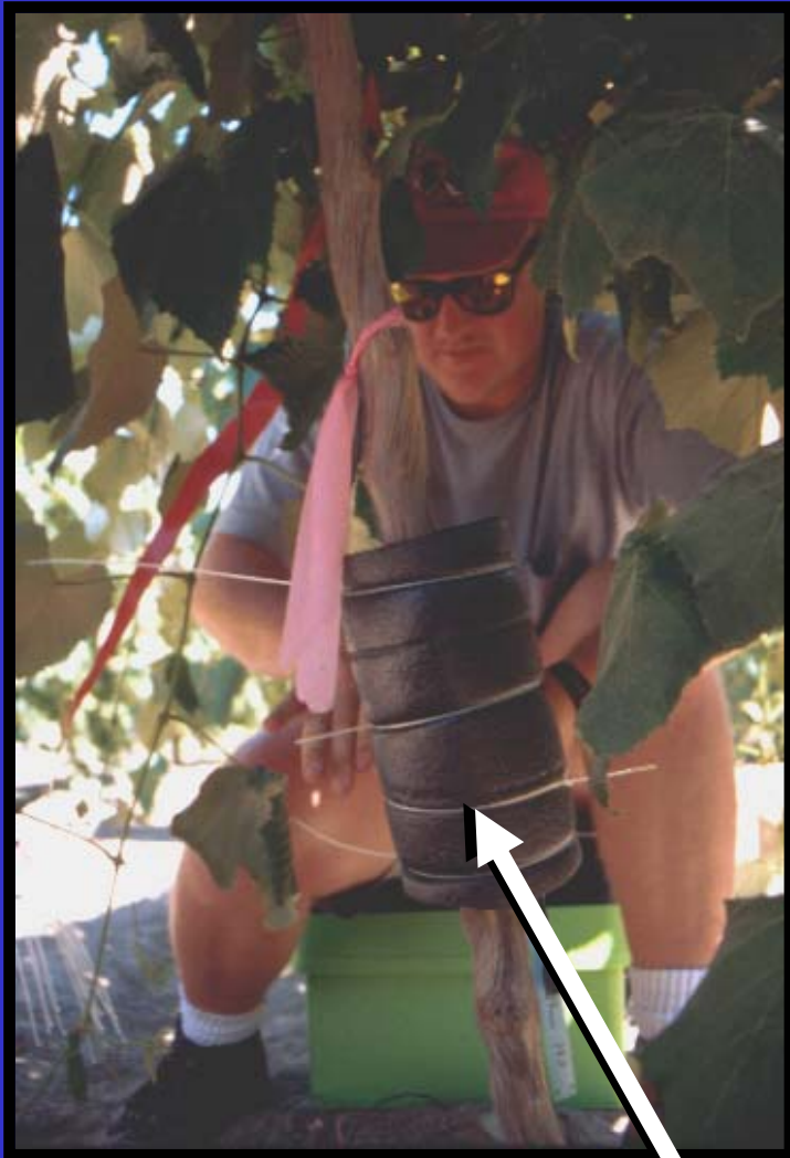
insulating sap gauge from environmental heating
